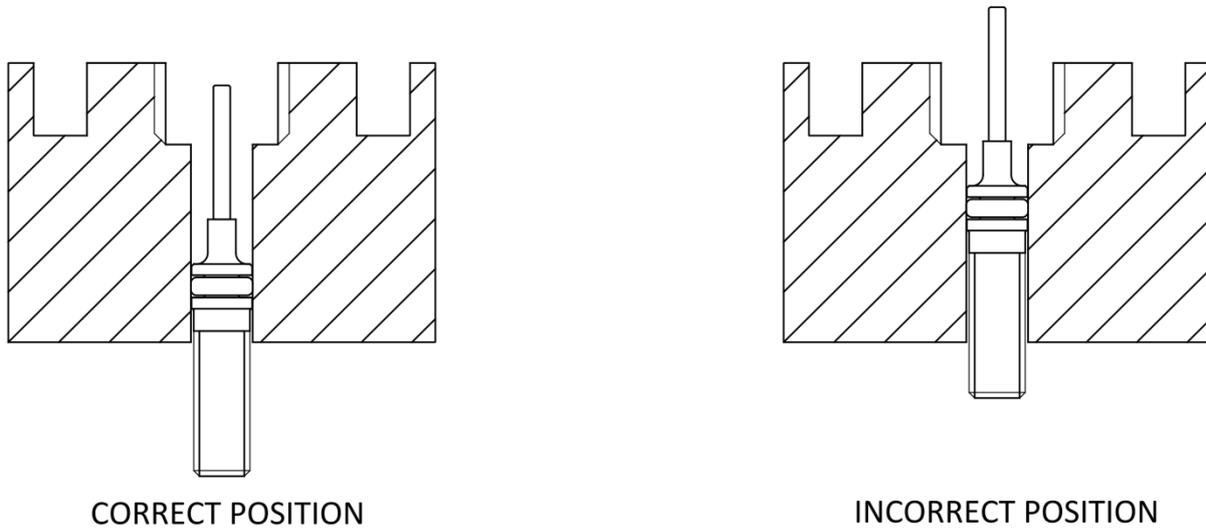
*Figure 5: Correct and Incorrect firing pin positions*
