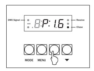
Now use the "**UP**" and "**DOWN**" buttons to select the program required from  $P:D \mid I \sim P: \mid E$ .
