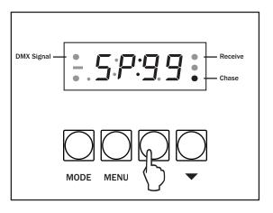
Now use the "**UP**" and "**DOWN**" buttons to select the chase speed required from  $5P:01 \sim 5P:99$ .
