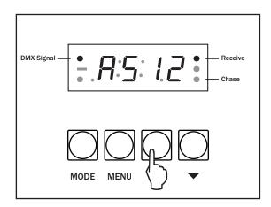
Now use the "**UP**" and "**DOWN**" buttons to set the required DMX address from **RDD I** ~ **R5 I2**.
