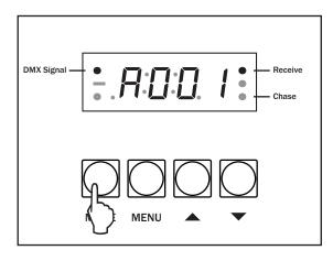
Press the **"MODE**" button on the front of the unit to show **ADD** I on the LCD display.
