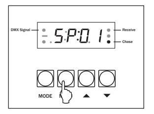
Press the "**MENU**" button on the front of the unit to show 5P:- - on the LCD display.
