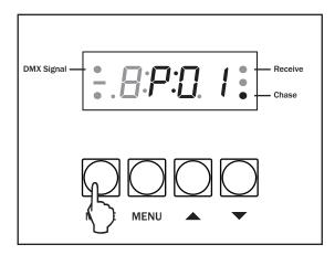
Press the "**MODE**" button on the front of the unit to show P: - - on the LCD display.
