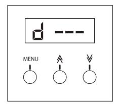
Press the "**UP**" or "**DOWN**" button so the display shows d - - -.
