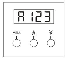
When the unit is powered up the unit will show the DMX address that the unit was last in before it was powered down. If the DMX address 123 was selected in the units last use the unit will display "A123".
