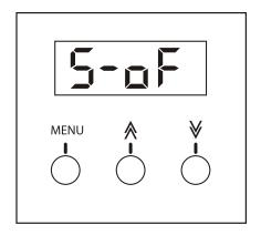
Press the "MENU" button to exit switch pack mode. In Switch pack on mode the output is on and the fixture will illuminate regardless of the DMX signal. In switch pack off mode the output is turned off and the fixture is controlled via the DMX signal. If the DMX level is less than 40% the fixture will blackout, above 40% the fixture will illuminate.
