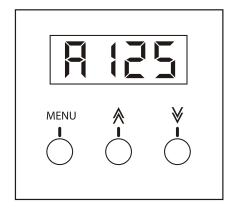
By using the "UP" or "DOWN" buttons the user is able to select the required DMX address. Once the DMX address is selected, it will be automatically stored into the units memory.
