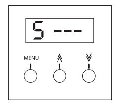
Press the "**UP**" or "**DOWN**" button so the display shows 5 - - -.
