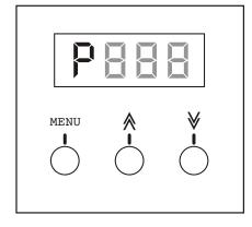
Use the "UP" or "DOWN" buttons to change the value between 00-100. Once the dimmer preset is selected it will be automatically stored into the units memory.
