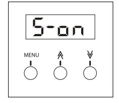
Press the "**MENU**" button to enter switch pack mode. Use the "**UP**" or "**DOWN**" buttons to change between 5 - an and 5 - aF.
