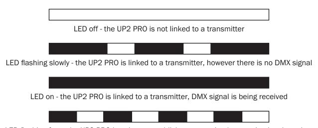
LED flashing fast - the UP2 PRO is trying to establish a connection/connection has been lost
