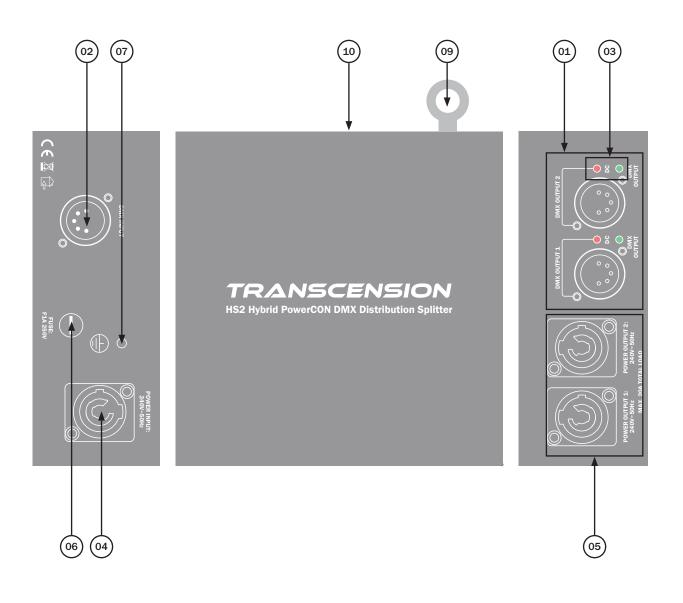
01 - 2 x 5-Pin DMX outputs 02 - 5-Pin DMX input 03 - DC/DMX output indicators
