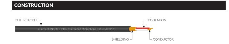
Professional quality, 2 core screened audio cable designed suitable for balanced microphone and line level connections within fixed installations. The small diameter cable is constructed from two oxygen-free cores, protected by a copper spiral screen and is finished with a black PVC outer jacket.
