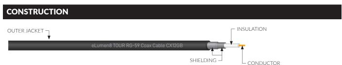
RG-59 style coaxial cable designed for analogue or HD-SDI video signals up to 12Gbps commonly used for high definition video signals in the event production sector. The cable is constructed from a single oxygen-free copper core, protected by both aluminium polyester foil and a tinned oxygen-free copper woven braid designed to reject interference. The cable is finished with a low memory, super flexible outer PVC jacket for the ultimate flexibility.
