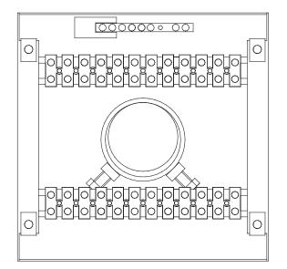
Fit the Terminal Brackets into the End Box using the Back Self-Tapping Screws. If a third Terminal Bracket is used this can be fitted after the wiring has been pulled into the tube.
