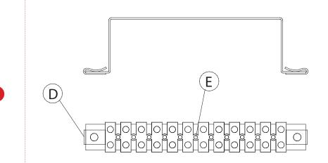
Fit the Earth Bar 'C' in the back of the End Box using the Black M3.5 x 12 screw and Lock Washer. Ensure one end of the Earth Bar fits into the small plate to prevent it rotating, and that the lock washer is fitted on the outside of the End Box.
