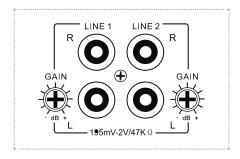
The line inputs will have an impedance of  $47k\Omega$ .
