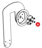
Install the positioning plate on the balance device (left and right).
