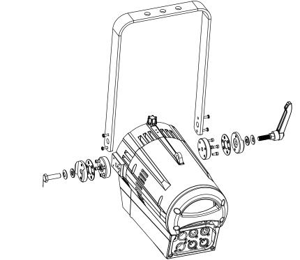
Remove the original bracket from the fixture.
