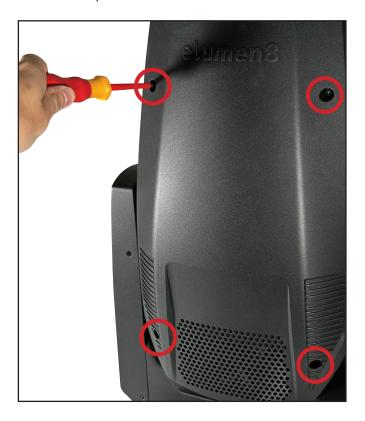
2) Use a Phillips head screwdriver to loosen the four screws on each side of the head casing. These are twist lock screws and do not come free of the casing.
