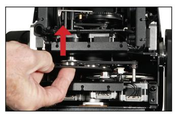
3) Push the gobo you are replacing up from underneath so it pops up.
