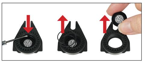
5) Place the gobo on a flat surface with the gear side down. Locate the tab of the spring clip using a precision pick (or similar) and push the spring clip inwards to release it and remove the spring clip. Carefully remove the gobo from the holder avoiding scratching the gobo. Install the new gobo and follow the previous steps in reverse order.
