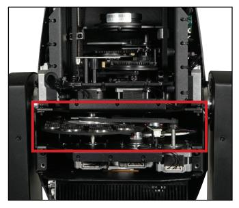
3) The replaceable gobo wheel is located here on the fixture. Manually spin the wheel to locate the gobo that will be replaced.
