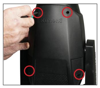
2) Use a Phillips head screwdriver to loosen the four screws on each side of the head casing. These are twist lock screws and do not come free of the casing.
