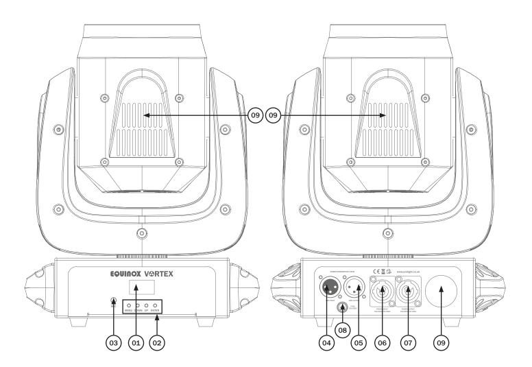
01 - OLED display 02 - Function buttons 03 - Microphone 04 - 3-Pin DMX input 05 - 3-Pin DMX output 06 - PowerCON input 07 - PowerCON output
