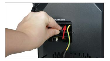
3) Carefully push the gobo holder you are wanting to replace upwards, away from the gobo wheel.
