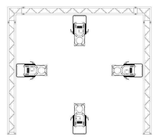
The Helix Scan XP 150W Scanner can be operated in a number of mounting positions as shown in the diagram above, hanging upside-down from the ceiling or truss, mounting sideways on truss or stood upright on a flat level surface. Always use a safety wire as an extra safety precaution to prevent damage/injury in the event a clamp fails (see the next page for clamp installation). Never use the carry handles for secondary attachments.
