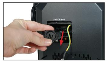
4) Pull the gobo holder out of the unit. Now you can remove the circlip, followed by the gobo from the gobo tray. Replace the gobo and fit the circlip back into the tray.
