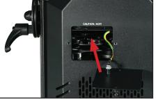
6) Move the gobo access door back into position over the gobo access slot, ensuring the earth wire isn't obstructing any mechanisms.
