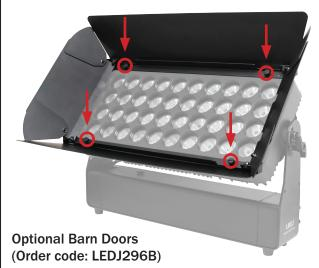
To fit the barn doors, place them over the front lens of the fixture and use the four thumbscrews located in each corner to tighten it to the fixture. The safety wire attached to the barn door can be clipped to one of the two holes in each of the side arms.
