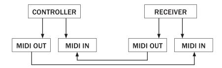
The controller sends and receives Note On and Note Off data via the 'Flash' buttons.
