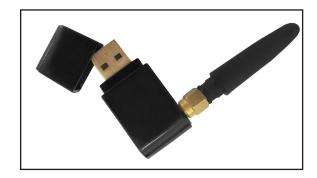
will scroll through the operating protocols. Once you have selected the chosen protocol, press and hold the button on the dongle for 3 seconds. The LED will illuminate white, then turn blue (transmit mode) or stay white (receive mode). The unit is now set in your chosen protocol.
