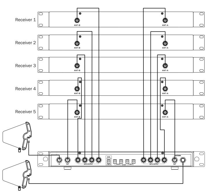
After installing the radio microphone receivers and ADS4 into a secure rack enclosure, using the short patch cables supplied, link the receivers individually taking care to avoid any cross wires between A and B channels. Additional ADS4 units maybe cascaded from the ANTENNA OUT link connectors.
