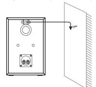
This allows the cabinet to be hung from a single screw that is firmly fixed into the wall.
