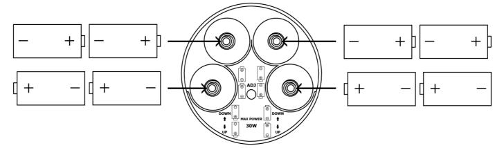
Plastic sleeves are provided for loading the D cells into the compartment in pairs. When loaded correctly, the compartment should appear as shown below.
