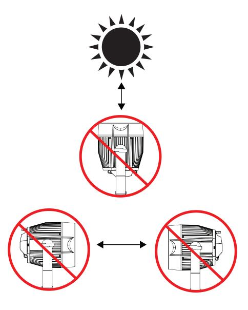
**NOTICE:** The maximum ambient operational temperature for this lighting fixture is *113° F (45° C)*. Do not place this lighting fixture in an environment where the temperatures exceed this value. This will allow the fixture to run at its best and help prolong the fixture life.
