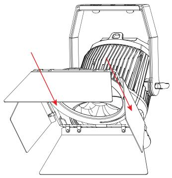
4. If desired, removed the barn door's included thumb screws, then slide the barn door into the slot in front of the gel frame.
