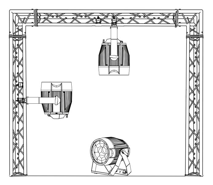
The unit is fully operational in three different mounting positions: hanging upside-down from the ceiling or trussing, sideways on trussing, or set on a flat level surface. Be sure this fixture is kept at least 12m (40ft) away from any flammable materials (decorations, etc). Always use and install a safety cable (not included) as a safety measure to prevent accidental damage and/or injury in the event the clamp fails. Never use the carrying handles for secondary attachment.
