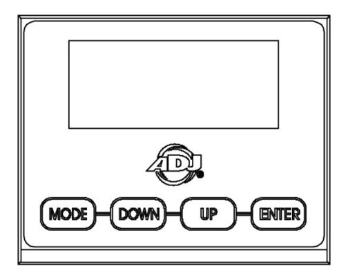
This device features two different settings for locking the keypad. Setting Lock to "ON" requires the user to simply press and hold the MODE button for 10 seconds to unlock the keypad.
