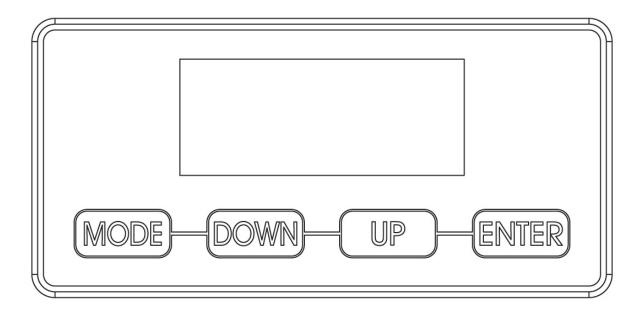
This device features two different settings for locking the keypad. Setting Lock to "ON" requires the user to simply press and hold the MODE button for 10 seconds to unlock the keypad.
