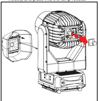
2. Loosen the screws on the head of the fixture and open the fixture head covers. Unplug the fan and loosen the screw that secures the safety cable.
