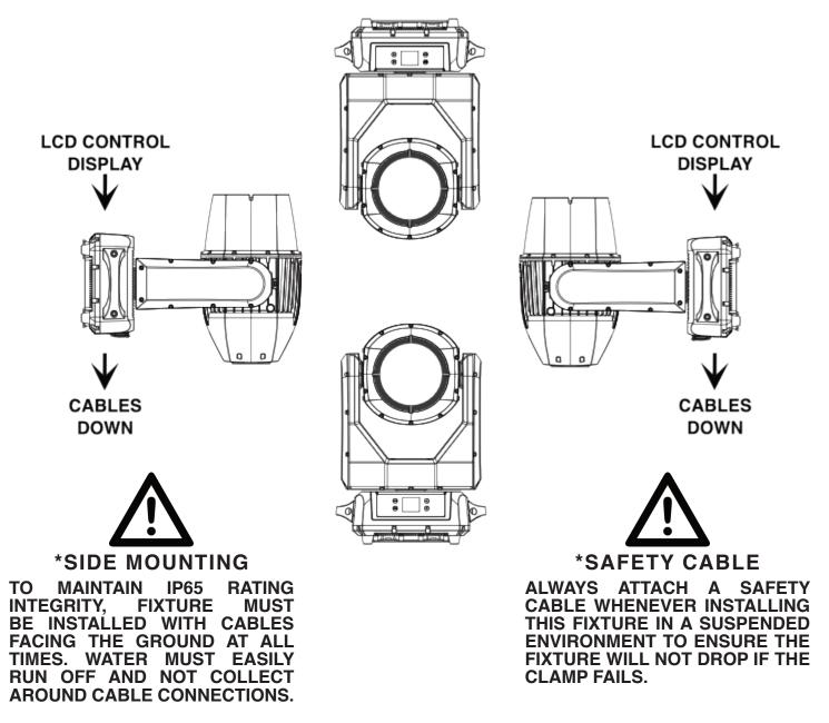
The Hydro Beam X12 is fully operational in three different mounting positions, hanging upside-down, mounted sideways on trussing, or set on a flat level surface. Be sure this fixture is kept at least 0.2m (7.9in.) away from any flammable materials (decoration etc.). Always use and install the supplied safety cable as a safety measure to prevent accidental damage and/or injury in the event the clamp fails (see next page). Never use the carrying handles for secondary attachment.
