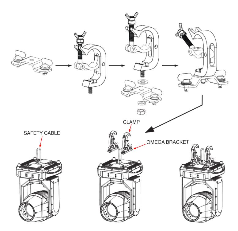
Screw one clamp via a M12 screw and nut into the Omega holder. Insert the quick-lock fasteners of the Omega holder into the respective holes of the adjustable mounting bracket. Tighten the quick-lock fasteners fully clockwise. Pull the safety-cable through the opening located on the bottom of the unit and over the trussing system or a safe fixation spot. Insert the end in the carabiner and tighten the safety screw.
