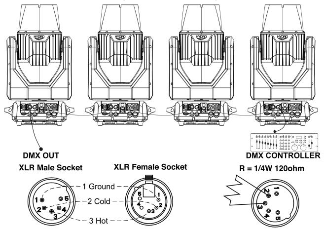
**Special Note: Line Termination.** When longer runs of cable are used, you may need to use a terminator on the last unit to avoid erratic behavior. A terminator is a 110-120 ohm 1/4 watt resistor which is connected between pins 2 and 3 of a male XLR connector (DATA + and DATA -). This unit is inserted in the female XLR connector of the last unit in your daisy chain to terminate the line. Using a cable terminator (ADJ part number Z-DMX/T) will decrease the possibilities of erratic behavior.
