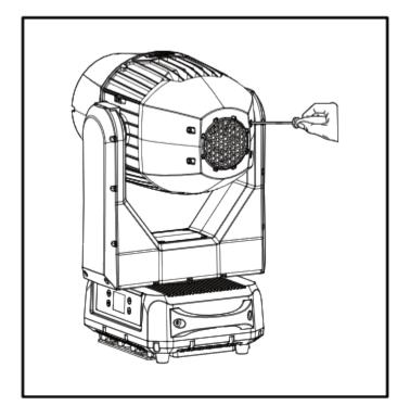
3. Loosen the screw that holds the lamp in place. Unplug the leads and lift the lamp out of its recess. Connect leads to the new lamp (same model), and place into the lamp recess.
