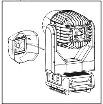
4. Reinstall the head panel, fastening it securely before reapplying power.
