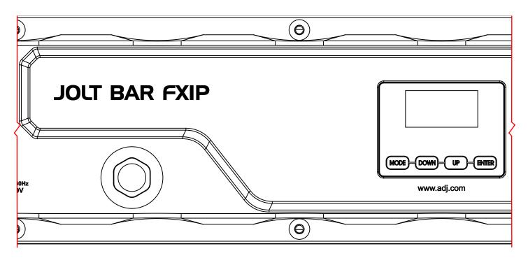
This fixture includes a display lock feature which automatically shuts off the display screen after a certain period of inactivity. This feature is OFF by default, which means that the display will always remain on regardless of inactivity, but can be configured to kick in after up to 10 minutes of inactivity. See the **System Menu** section of this manual for details on how to configure this setting.
