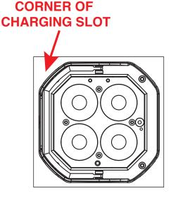
4. Place an ADJ Mirage Q IP Black device in any of the device slots in the flight case. Up to 6 devices can be accommodated. The charge indicator located beside the power ports will illuminate to indicate that your device is charging. *It is strongly recommended to leave the case lid open during charging.*
