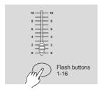
2. Tap the Flash button numbered from 1-16 to assign MIDI IN channel 1-16, the relevant channel LED lights indicating MIDI IN channel is set.
