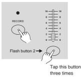
1. Tap the Flash button 2 three times while holding down the Record button, the Segment Display reads "CHO" indicating MIDI OUT channel setup is available.
