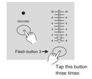
Tap the Flash button 3 three times while holding down the Record button, the Segment Display reads "IN" indicating the controller is ready to receive MIDI file dump.
