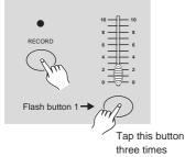
1. Tap the Flash button 1 three times while holding down the Record button, the Segment Display reads "CHI" indicating MIDI IN channel setup is available.
