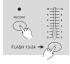
7. Press a Flash button between 13-24 while holding down the Record button. All LED will flash indicating the scenes have been programmed into memory.
