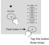
Tap the Flash button 4 three times while holding down the Record button, the Segment Display reads "OUT" indicating the controller is ready to send a file.
