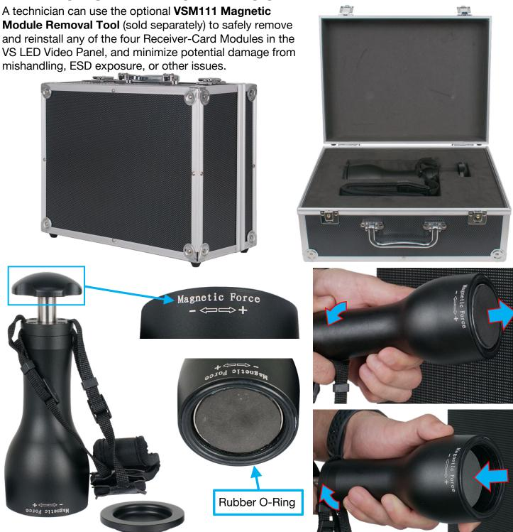
The percieved "Magnetic Force" is relative to the distance the magnet is from the surface. Turning the knob clockwise, in the "+" direction, advances the magnet, moving it closer to the front, and turning it counterclockwise, in the "-" direction, retracts the magnet, moving it away from the front.
