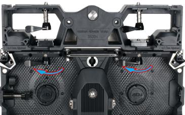
Release latch to hold the vertical connector. To lock, twist vertical connector lever to the left.
