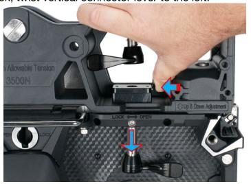
To unlock the vertical connector, rotate lever to the right (counter-clockwise), then press springloaded locking latch inward. The vertical connector will drop open.
