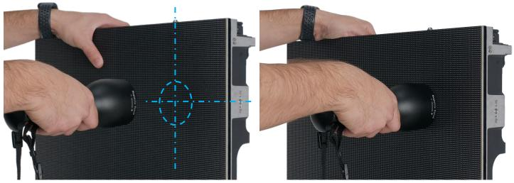
Locate the center of selected LED moduleto be removed (1 of 4), and place the O-Ring of the Magnetic Module Removal Tool against its surface.
