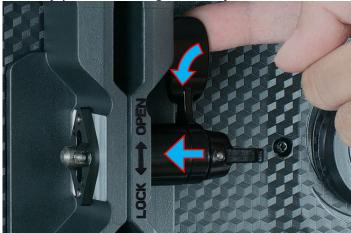
Rotate handle down (counterclockwise) to cinch horizontal tab-keyed connector.
