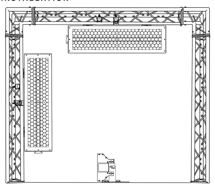
The unit is fully operational in three different mounting positions: hanging upside-down from the ceiling or trussing, sideways on trussing, or set on a flat level surface. Be sure this fixture is kept at least 9.8 ft (3m) away from any flammable materials (decorations, etc). Always use and install a safety cable (not included) as a safety measure to prevent accidental damage and/or injury in the event the clamp fails. Never use the carrying handles for secondary attachment.
