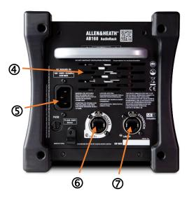
**Vents** Ensure good ventilation at the sides and back of the rack. Avoid obstruction of vents while operating. Avoid dirt or liquid ingress.
