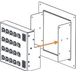
**Flush mounting in a wall** Use the mounting frame AA11504 in the orientation shown below. Align the threaded inserts on the sides of the DT164-W with the frame, and secure the unit in place with the 6x M4 6mm T20 screws provided. Connect the power and Cat5 cable/s, then fix the assembly to the wall using appropriate fixings or screws for the type of wall.
