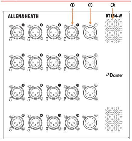
① Input sockets Balanced XLR mic/line inputs with +48V Phantom Power indicator. The preamps are built into the DT164-W and their Gain, Pad and +48V are controlled from the network.
