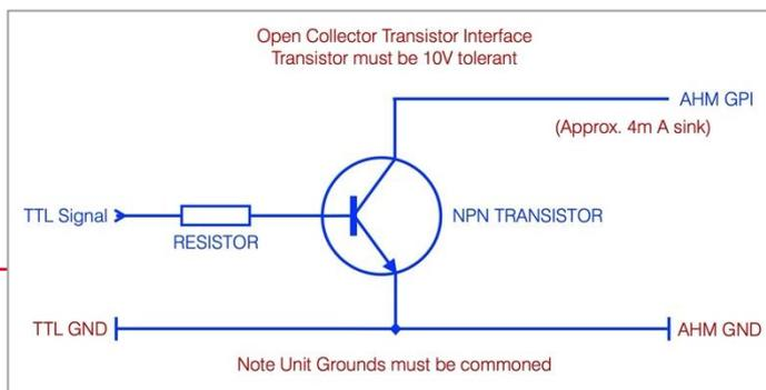
A transistor can be an alternative to a relay module for the switching. In this case, a 10kOhm resistor and a BC547 or 2N222 transistor can be used.
