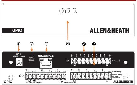
O **DC input -** The unit can be powered by the supplied AC/DC adapter or alternatively via Cat5 cable when connected to a PoE source.
