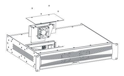
• Replace the cover and secure in place using the 4x screws.
