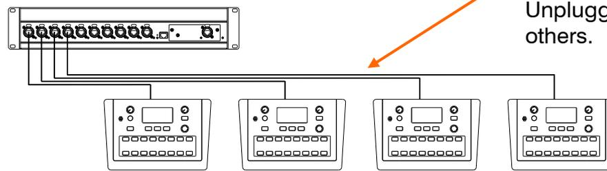
Each ME mixer is powered over its Cat5 cable. You do not need to use its power unit. Unplugging one ME mixer does not affect the others.
