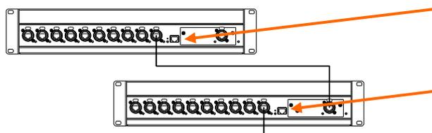
Connect any Output port from the first ME-U to the Input port of the next ME-U. Use the **first ME-U** hub Setup Application to set its names and stereo links. Tick the iLive Source Mode if connecting an iLive system. Use the **next ME-U** hub Setup Application for received names and stereo links. Make sure you untick its iLive Source mode.
