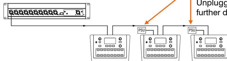
The first ME mixer in the chain gets PoE to power it over its Cat5 cable. Use external power units for the others in the chain. Unplugging one ME mixer disconnects others further down the chain.
