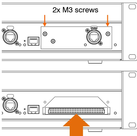
Slide card in to plug into connector
