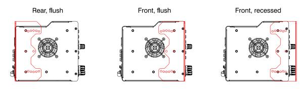
The entire unit can be angled by  $\pm 7.5^{\circ}$  or  $\pm 15^{\circ}$  by turning the ears about the centre fixing. Note that when mounting at an angle in a rack, more that 4U space may be required.
