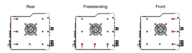
Flush or recessed positions are available when mounting straight (0°), with the rack strip or surface parallel to the front, rear or base of the SQ-Rack.
