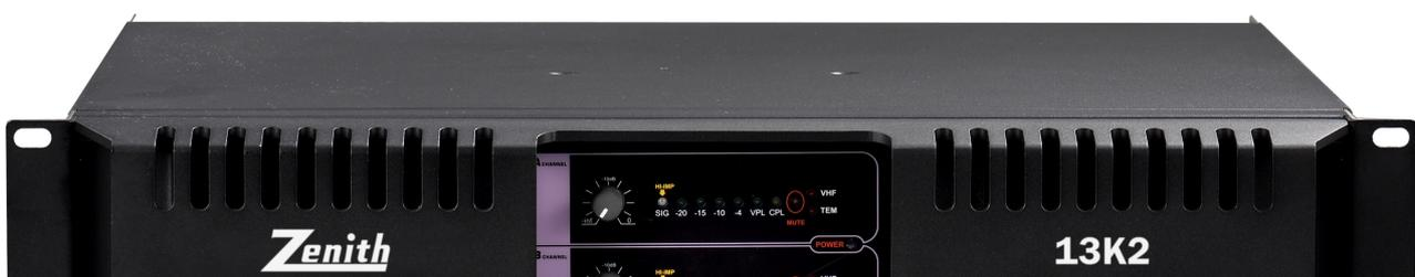
The amplifier's front panel presents the performance and fault condition indicators, power and remote switches, and a removable dust-filter cover. Level potentiometers provide individual attenuation for the amplifier channels. Range is 0dB to - infinity. (The 12 o'clock position indicates -10dB attenuation.)
