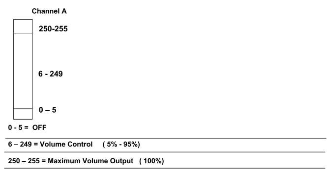
The ICE Low Fog Machines has onboard DMX control. Currently it uses one channel to control volume output operation. Each channel has a value range of 0 to 255. Timer functions such as duration and interval can be programmed using the DMX controller or the DMX control software being used by lighting and effects operator.
