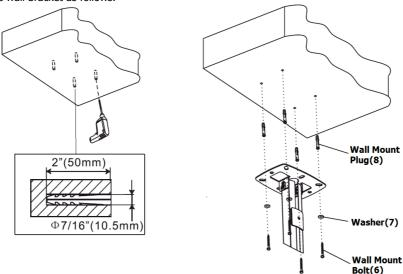
For plaster ceiling installation first you need to find out where the wood stud is behind the plastered ceiling using a stud finder. Then work out the required position, hold the bracket against the ceiling and use pencil to mark where the mounting holes will be. Use an electric drill to drill a hole that is around 3mm in diameter and 50mm deep. Install the wall bracket as follows.
