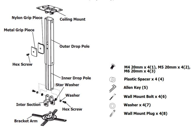
For this installation you will also require a pencil, tape measure, electric drill, stud finder and a Philips (cross) screw driver.
