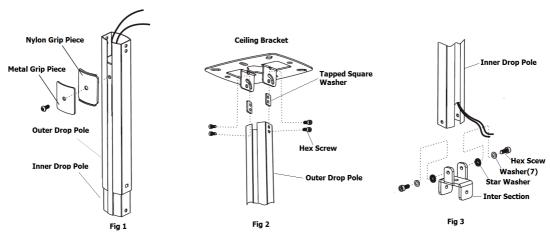
Step 2 – Fixing bracket to the ceiling
