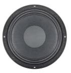
The MBX series mid-bass woofers from B&C Speakers offer acoustic designers a new range of high efficiency, wide bandwidth alternatives that are not currently available in the B&C range. These full-featured transducers incorporate lightweight neodymium motors, inside/outside wound copper clad aluminum wire voice coils, weatherproof impregnated paper cones, and a symmetrical inductance profile. The MBX Series is especially well suited for two-way loudspeaker enclosures.
