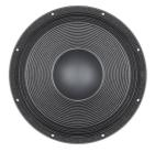
This next evolution subwoofer uses a new, longer, four layer aluminum voice coil. The result is less heat, more energy in the gap, higher sensitivity, higher power handling, lower distortion and better overall performance. The 15DS100 features a 37mm long, 4 inch diameter (100mm) Copper Clad Aluminum Wire voice coil. With a 1500watt AES power rating, 96.8 dB sensitivity, and over 14.0mm of Xvar, this high energy subwoofer is a significant step forward from similar models in the B&C range.
