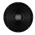
This next evolution subwoofer uses a new, longer, four layer aluminum voice coil. The result is more energy in the gap, higher sensitivity, lower distortion and better overall performance. The 15DS115 features a 40mm long, 4.5 inch diameter (116mm) Copper Clad Aluminum Wire voice coil. With a 1600watt AES power rating, 96 dB sensitivity, and over 14 mm of Xvar, this high energy subwoofer is a significant step forward from similar models in the B&C range.
