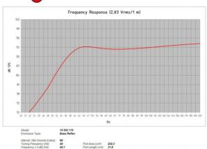
nited Maximum SPL at 1 meter (dB): 122,6 equal to 695,2 Watts (Bass Band Power Rating) ed Maximum SPL at 1 meter (dB): 126,0 equal to 1500,0 Watts (filled Band Power Rating)
