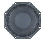
The FMB series mid-bass woofers from B&C Speakers offer acoustic designers a new range of high efficiency, wide bandwidth alternatives that are not currently available in the B&C range. These full-featured transducers incorporate lower cost ferrite motors, inside/outside wound copper clad aluminum wire voice coils, weatherproof impregnated paper cones, and a symmetrical inductance profile. The FMB Series is especially well suited for two-way loudspeaker enclosures.
