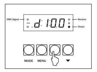
Now use the "UP" and "DOWN" buttons to select the chase light output intensity required from  $d \Box \Box \Box \Box \sim d \Box \Box \Box$ .
