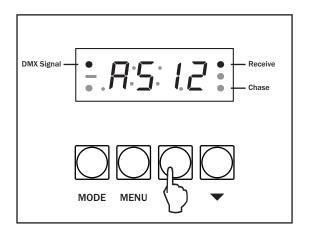
Now use the "UP" and "DOWN" buttons to set the required DMX address from  $RDD I \sim R5 I2$ .
