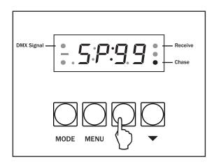
Now use the "**UP**" and "**DOWN**" buttons to select the chase speed required from  $5P:\square I \sim 5P:\square S$ .
