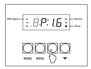
Now use the "UP" and "DOWN" buttons to select the program required from  $P: \square I \sim P: I \subseteq I$ .
