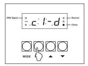
Press the "MENU" button again to show  $c \cdot l - d$  (channel 1) on the LCD display.
