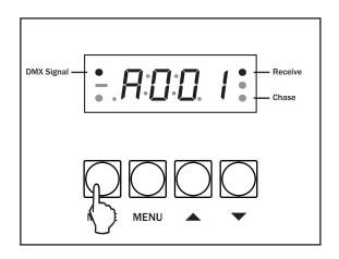
Press the "MODE" button on the front of the unit to show  $\Pi \square \square I$  on the LCD display.
