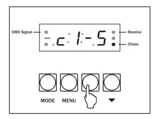
Now use the "**UP**" and "**DOWN**" buttons to set whether each channel is a dimmer ( d) or switch ( 5).
