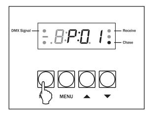
Press the "**MODE**" button on the front of the unit to show P: -- on the LCD display.
