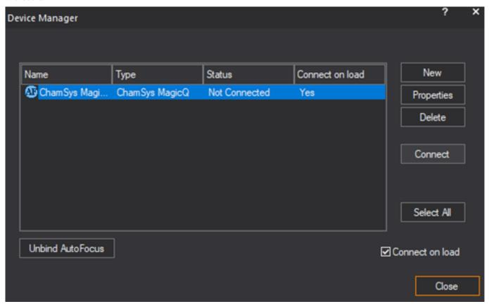
The universes in WYSIWYG must be bound to the ChamSys MagicQ device in order for communication to occur with MagicQ. Select ChamSys MagicQ and click on *Properties* to setup universe mapping.
