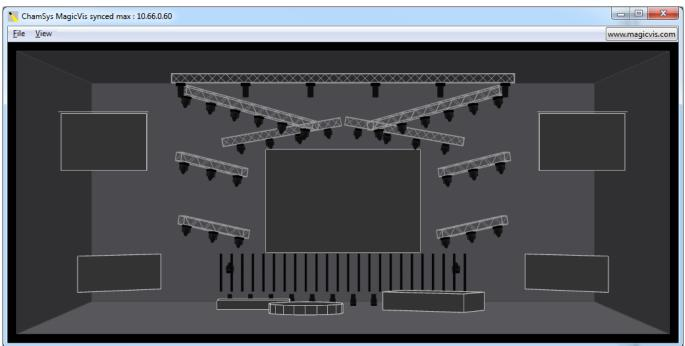
Initially the title bar in MagicVis will show **searching for consoles**, then **trying to connect** once it has found a console. Once a connection has been made with the console then it will change to say **waiting sync**. Once the show data has been transferred over the connection from the console to the MagicQ vis application then it will change to say **synced**.
