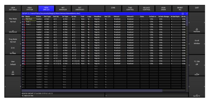
To enable output of channel data select the DMX IO VIEW in the Setup Window. This window enables modification of the inputs and outputs for all the universes. MagicQ consoles support DMX directly from the console or via an external Ethernet to DMX convertor. On MagicQ PC or Mac you can output via USB to DMX interfaces (such as MagicDMX) or via DMX outputs from the Wings.
