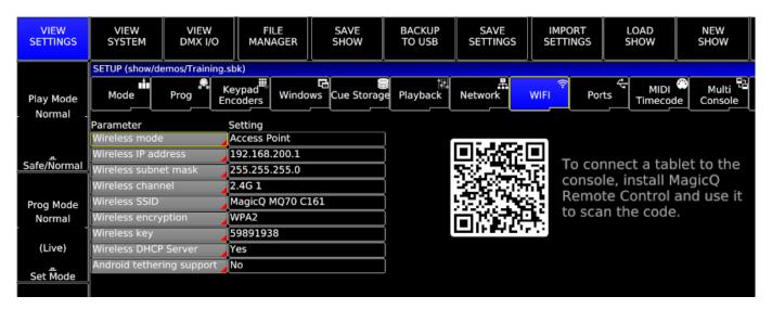
Wireless mode needs to be set to "Access Point" or "Access Point (Hidden SSID)".
