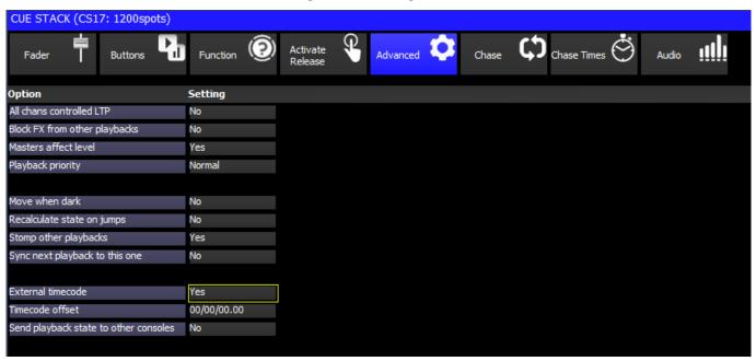
Time code can be triggered from an external timecode source using the MagicQ MIDI/Timecode module, or it can run from the internal time code source. To control a Cue Stack using external timecode set the "External timecode" option in the Cue Stack options.
