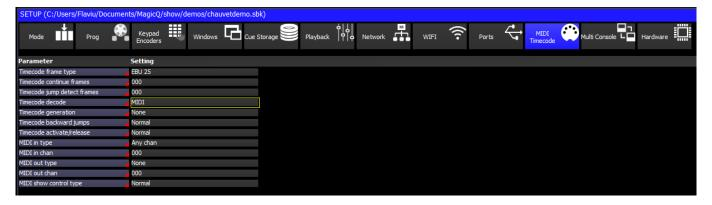
Set the Timecode Decode to LTC, MIDI, Art-Net or Internal MagicHD depending on the timecode source.
