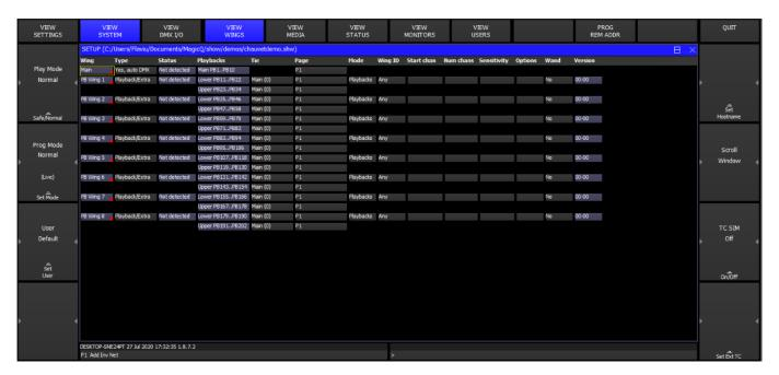
To enable the Scene Setter in MagicQ software, set one of the Wings in Setup, View System, View Wings to "Remote Panels".
