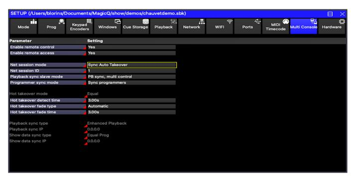
The first console to start becomes the Master. In Setup, View DMX I/O, Take Control and Release Control can be used to swap which console is the Master at any time.
