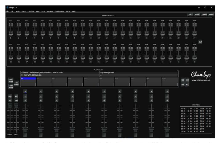
In this mode the console simply operates as a 48 channel traditional theatre console with 48 dimmers patched on Universe 1 at channels 1 through 48.
