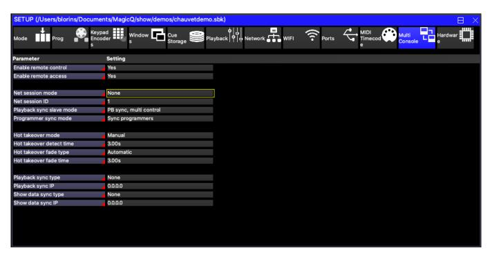
Configure the master console by setting the multi console setting "Show data sync type" to "Master Prog".
