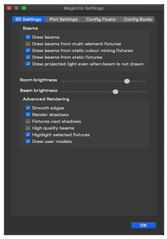
On systems with lower power graphics cards which are using a lot of LED heads we recommend to turn off drawing of LED Beams.
