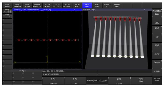
FOCUS LINE allows easy creation of even stage washes but it can also be used to create gobo washes on walls and scenery or ACL style beam focuses. Use the Fan menu to change how the beams are distributed along the line. To create a symmetrical ACL style look first focus one side of heads, then select the other side, select FOCUS LINE again and press Encoder E, *Mirror Line*. This will mirror the line over the centre line of the stage so the look is symmetrical.
