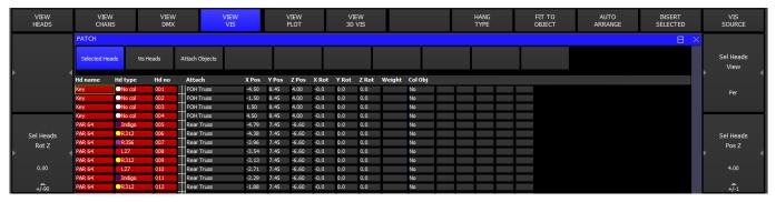
In *Selected Heads*, all the visualiser heads for the currently selected heads will be shown in the list. Heads are selected as usual using groups or direct from the keypad. In this view the encoders and soft buttons will apply changes to all the visualiser heads for the selected heads.
