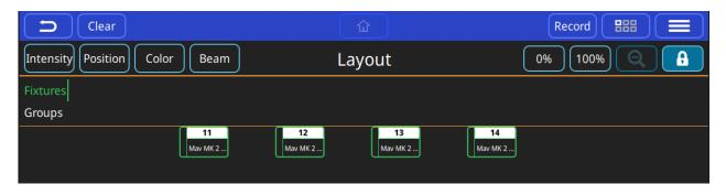
The larger fader on the left controls all currently selected instruments. You can also modify individual instruments by selecting them in this window.
