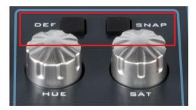
The [DEF] button (Default) will bring your colour mixing lights back to their Default colour with one touch of the button. The Default colour is normally white. You can change the default colour of any colour mixing fixture by simply saving that new colour to the first colour palette (the one that has the word 'Default' in green) in the colour window.
