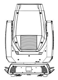
2. Remove both head covers by removing 8 Phillips-head <sup>1</sup>/<sub>4</sub>-turn screws.
