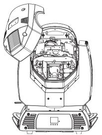
4. Remove the 2 wires connected to the lamp by the spade terminals.Using the lamp base, push the lamp to the left against the spring clips located on the left.
