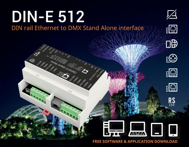
DIN is the ideal DMX stand alone interface for installation in electrical DIN cabinets with DIN rails. The USB to DMX stand alone Ethernet DMX device can control from 512 to 2048 channels on 1, 2 or 4 DMX universes.
