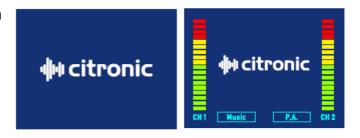
Pressing the DSP/MODE rotary selector (6) will open up the menu, rotating the selector will step through the options. Within each sub menu, selecting BACK will return to the main menu.
